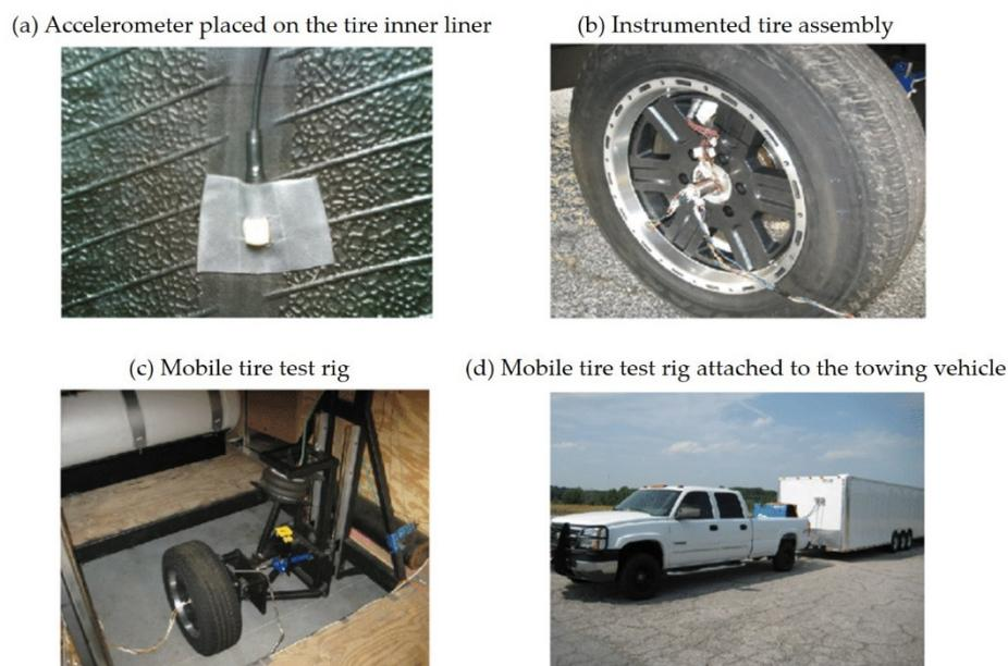
**Figure 11.** Full-scale application of a smart tire system and its components [87].
