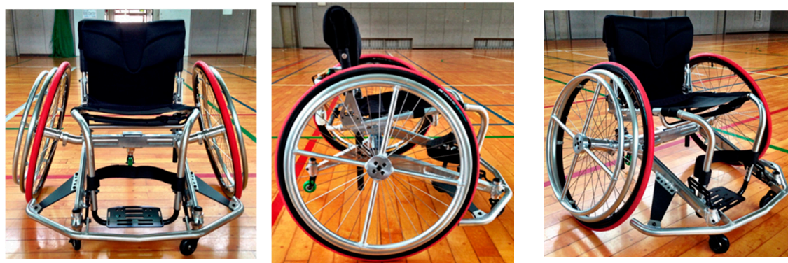
Figure 3. The outward appearance of new wheel-chair for sports competition which can drive straight by one-hand operation.
