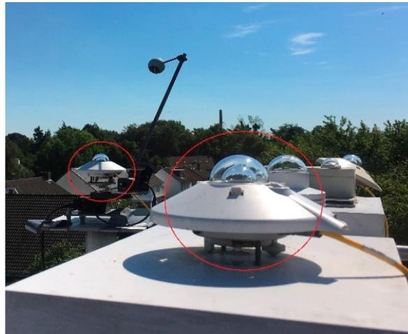
**Figure 1.** Photo of a pyranometer [6].
