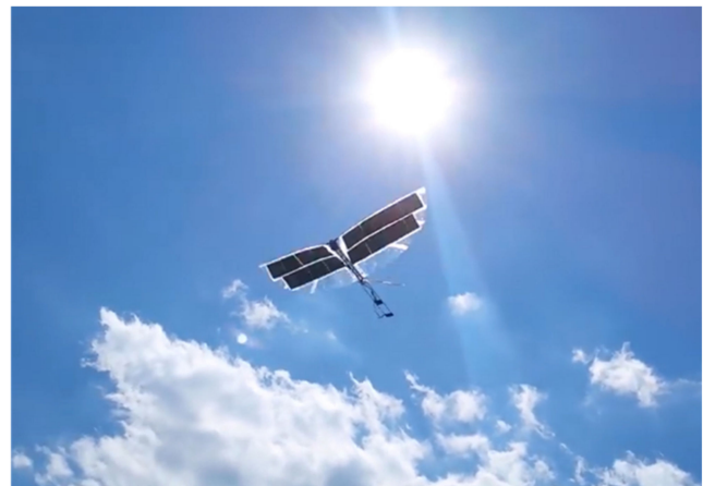
Figure 12. Robo Raven III: Solar-powered flapping wing flight using flexible solar cells integrated into wings.
