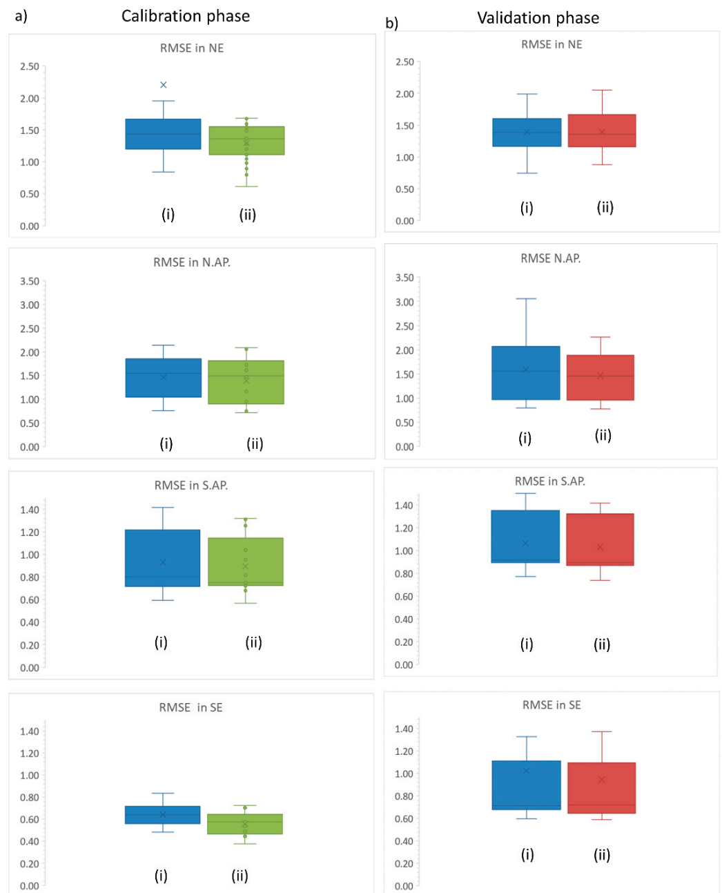
Figure 5. RMSE results calculated from predicted and simulated discharges using a priori and calibrated parameters in calibration (panel (a) of the Figure) and validation (panel (b) of the Figure). In panels (a,b), the boxplots (i) used the a priori parameters and the boxplot (ii) used the calibrated parameters. NE stands for north east, N.AP. stands for North Appalachian, S.AP. stands for south Appalachian, SE stands for south east.
