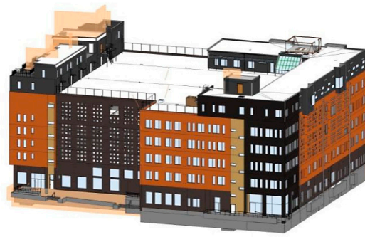
Figure 6. Industry Foundation Classes (IFC) model shown in Revit (Source: NCC Company).
