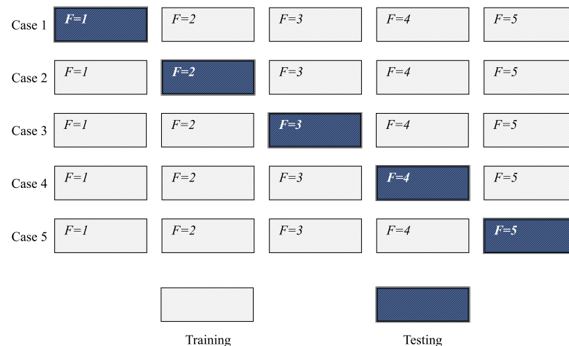
Figure 10. A schematic representation of the five-fold cross-validation procedure.
