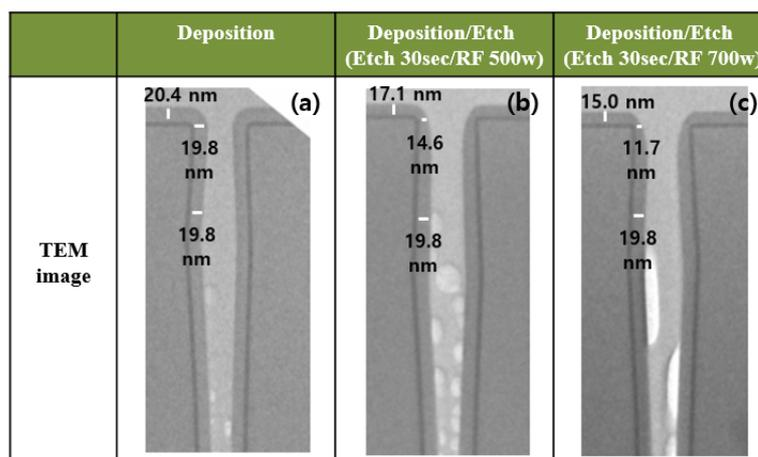
**Figure 11.** Analysis of the influence of etching in the pattern. (a) Pattern image when deposited only. (b) Pattern image when deposited by increasing RF power (500 w). (c) Pattern image when deposited by increasing RF power (700 w)
