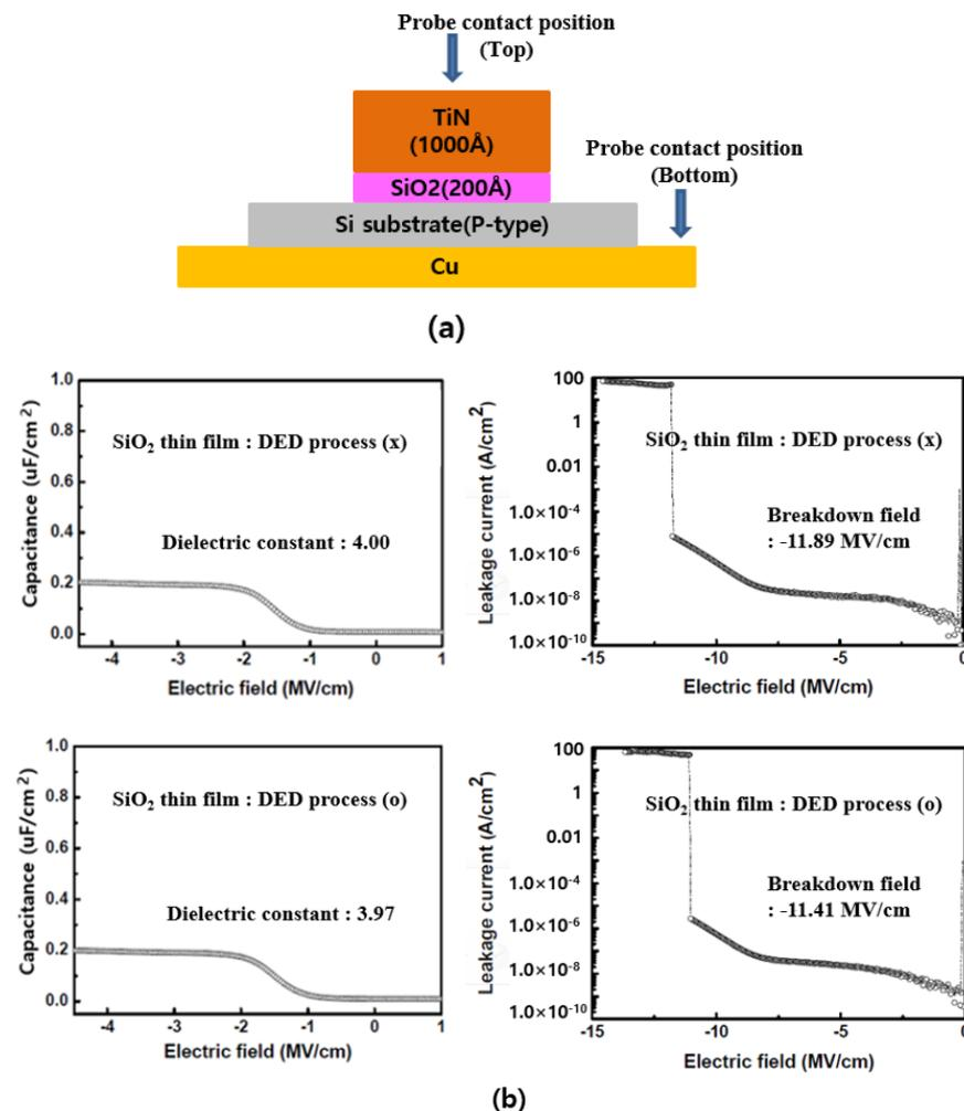
**Figure 10.** (a) Fabrication of a MOCAP device for C-V and I-V characterization and (b) dielectric constant and breakdown field of the deposited SiO<sub>2</sub> thin films.
