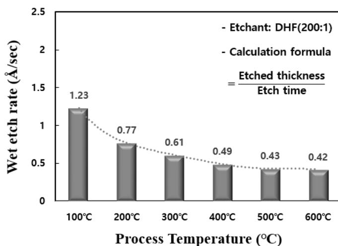
Figure 2. Wet etch rate characteristics of SiO<sub>2</sub> thin film at various process temperatures.
