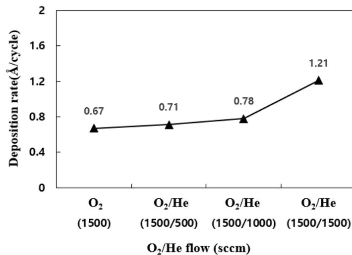
**Figure 6.** Reactant gas O<sub>2</sub>: deposition rate trend according to He flow rate.
