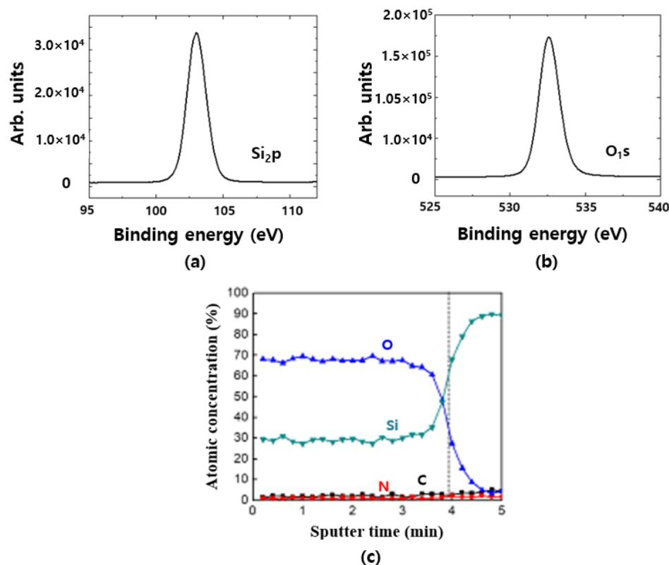
**Figure 5.** XPS spectra of SiO<sub>2</sub> are also shown: (a) Si<sub>2p</sub> and (b) O<sub>1s</sub>. (c) Deposited thin-film composition analysis.
