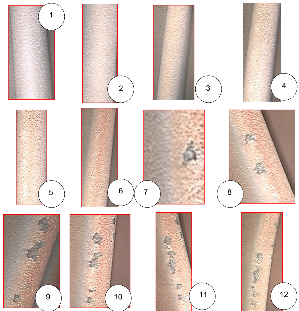
Figure 9. Deterioration of blade 13 (APS + SLURRY) observed at successive inspections (1-12).
