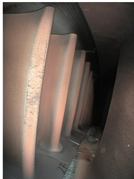
Figure 5. C-coated blade 27 viewed through the borescope at the 12th inspection.
