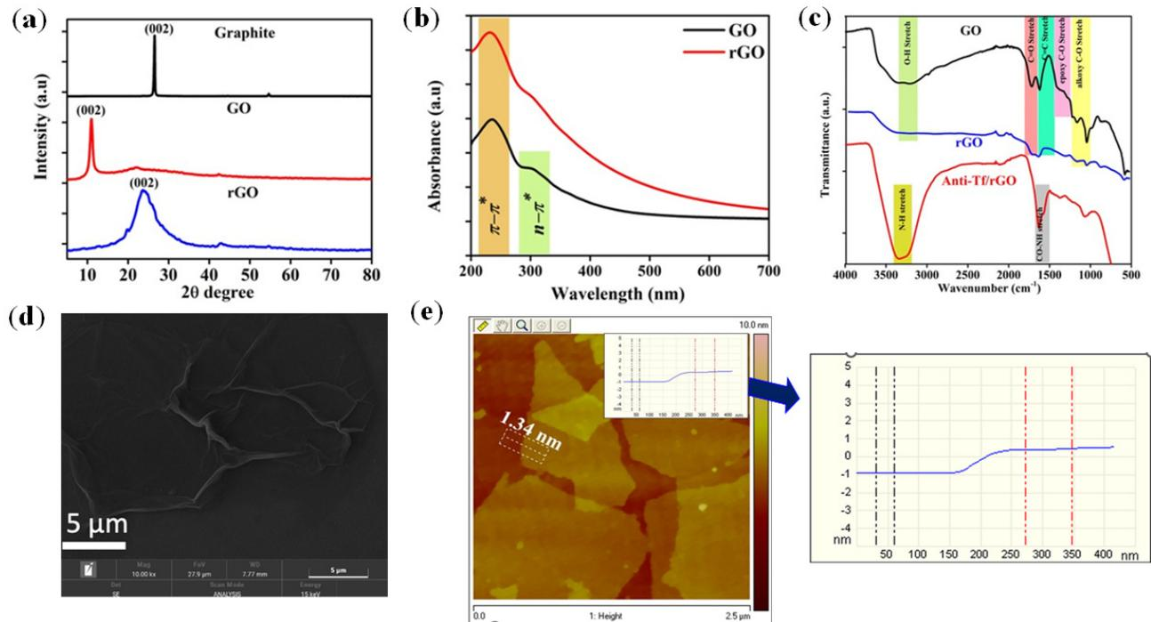
**Figure 1.** (a) X-ray diffraction pattern of GO, graphite, and rGO; (b) UV–Visible spectra of prepared GO and rGO; (c) FTIR spectroscopy of GO, anti–Tf/rGO, and rGO; (d) SEM image of GO; (e) AFM image of GO.
