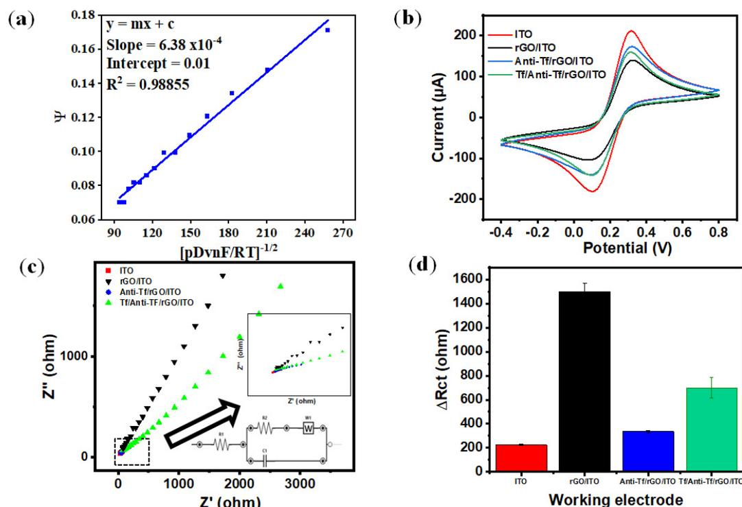
**Figure 3.** (a) Plot of  $\Psi$  vs. square root of  $pDvnF/RT$  for rGO/ITO; (b) CV of all modified electrodes; (c) EIS response of all modified surfaces with the equivalent circuit model; inset shows a zoomed-in view of all responses; (d) comparative histogram of the Rct values of all electrode surfaces, highlighting the increased resistance of the final surface caused by insulation on the electrode surface.
