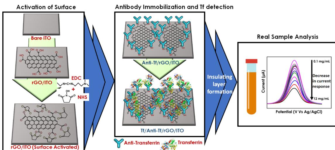
**Scheme 1.** Fabrication and Tf detection strategy using anti-Tf/rGO/ITO immunosensor.
