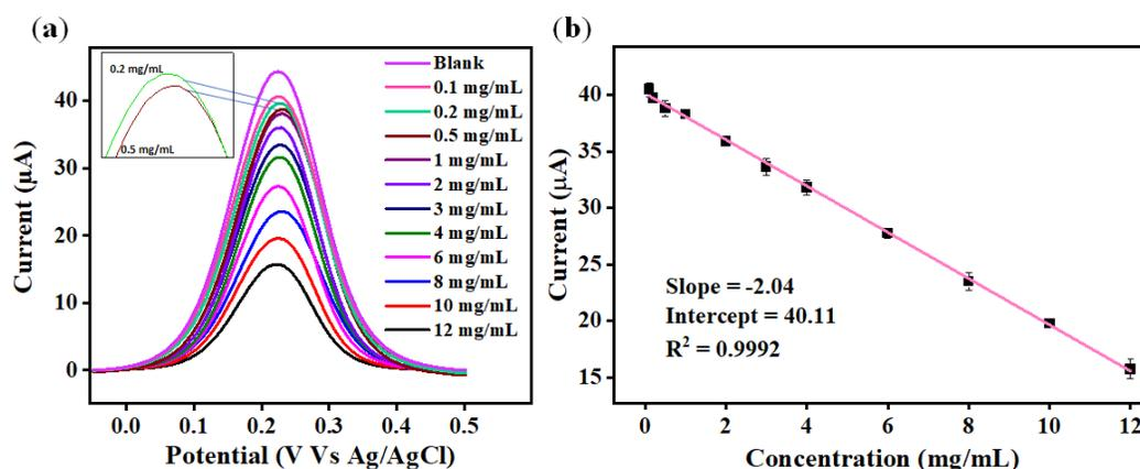
**Figure 4.** (a) DPV curves depicting the responses of the anti-Tf/rGO/ITO immunosensor to different concentrations of Tf; (b) calibration curve showing the relationship between the response current of the immunosensor and the varying concentrations of Tf antigen.
