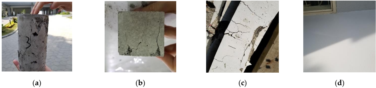
Figure 3. (a) Dataset from cylindrical concrete specimen; (b) dataset from mortar specimen; (c) dataset from beam specimen; (d) dataset from concrete wall.
