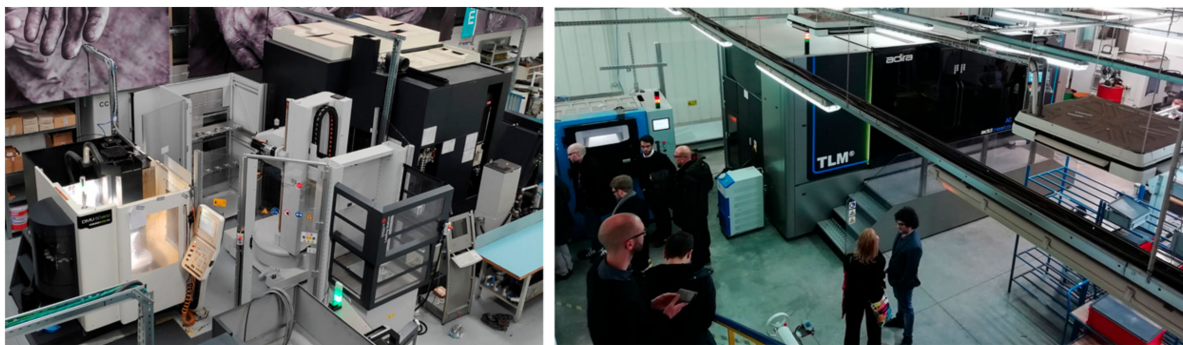
Figure 13. Final demonstrations of the Hybrid SLM production cell at POLY-SHAPE (right) and post-processing cell for machining SLM parts in RAMEM (left).
