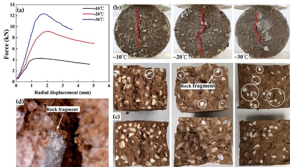
**Figure 6.** Failure patterns of FSRMs under Brazilian testing: (a) radial force–displacement curves; (b) failure patterns; (c) the rock fragments in the tensile cracks; (d) fracture morphology of a rock fragment.
