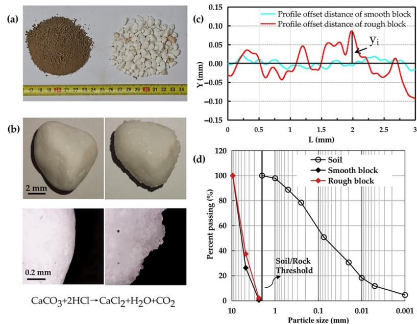
**Figure 1.** Materials: (a) soil and rock block particles; (b) surface morphology of rock blocks; (c) profile offset distance of rock blocks; (d) particle distributions.
