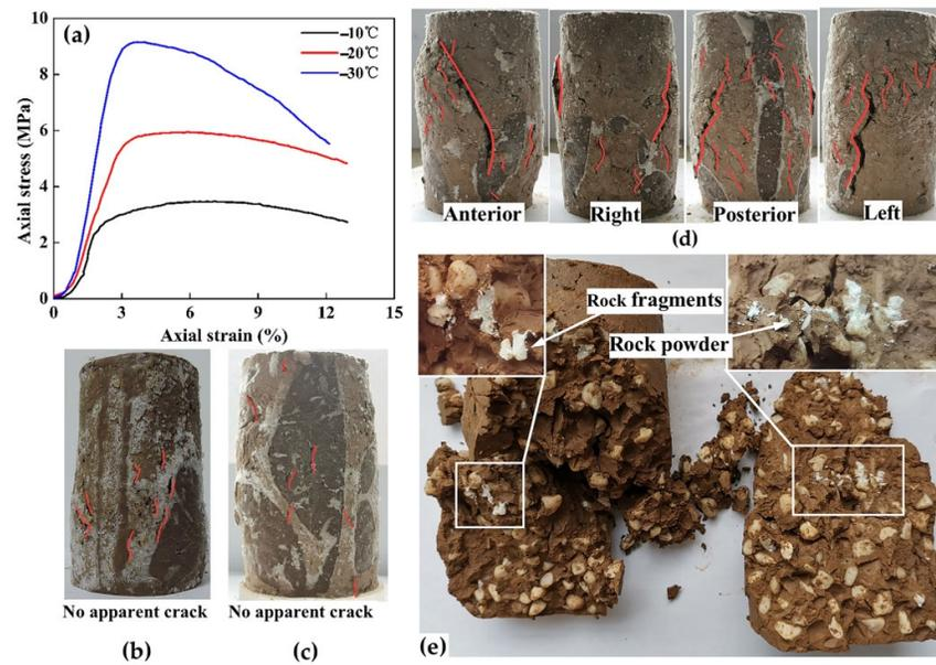
**Figure 5.** Failure patterns of frozen soil–rock mixtures (FSRMs) under uniaxial compression: (a) stress–strain curves; (b) failure pattern of the FSRM at  $-10\text{ }^{\circ}\text{C}$ ; (c) failure pattern of the FSRM at  $-20\text{ }^{\circ}\text{C}$ ; (d) failure pattern of the FSRM at  $-30\text{ }^{\circ}\text{C}$ ; (e) rock block fragments in the internal crack of the FSRM at  $-30\text{ }^{\circ}\text{C}$ .
