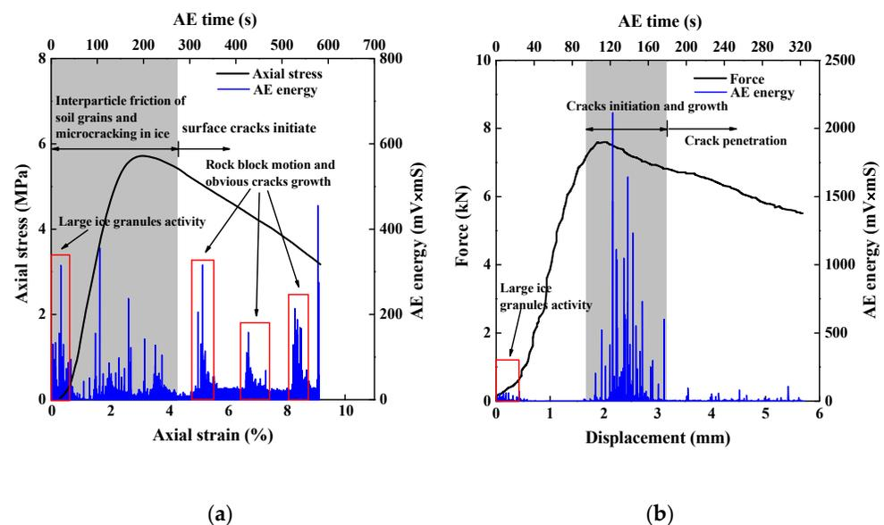
**Figure 7.** AE characteristics of FSRMs: (a) uniaxial compression test; (b) Brazilian test.
