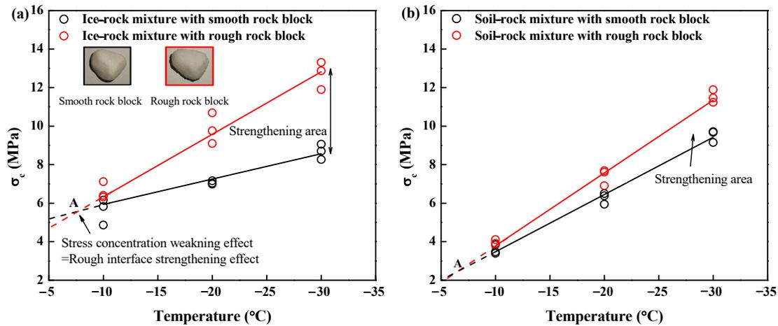
**Figure 12.** Relationship between the uniaxial compression strength (UCS) and the frozen temperature (a) ice–rock mixture; (b) soil–rock mixture.
