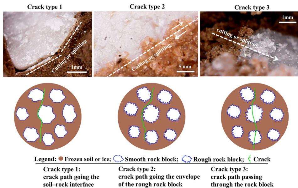
**Figure 15.** Three possible crack propagation types for FSRMs.
