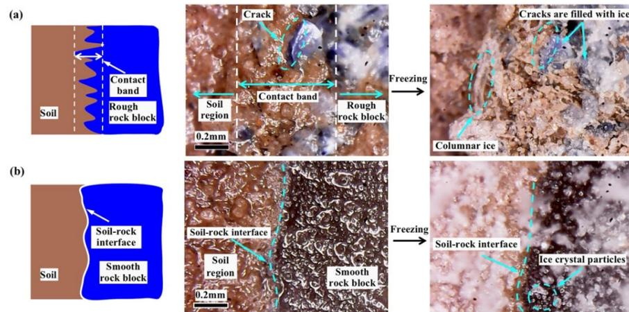
**Figure 11.** The morphology of soil–rock interface (contact band) before and after freezing: (a) rough soil–rock interface (contact band); (b) smooth soil–rock interface.
