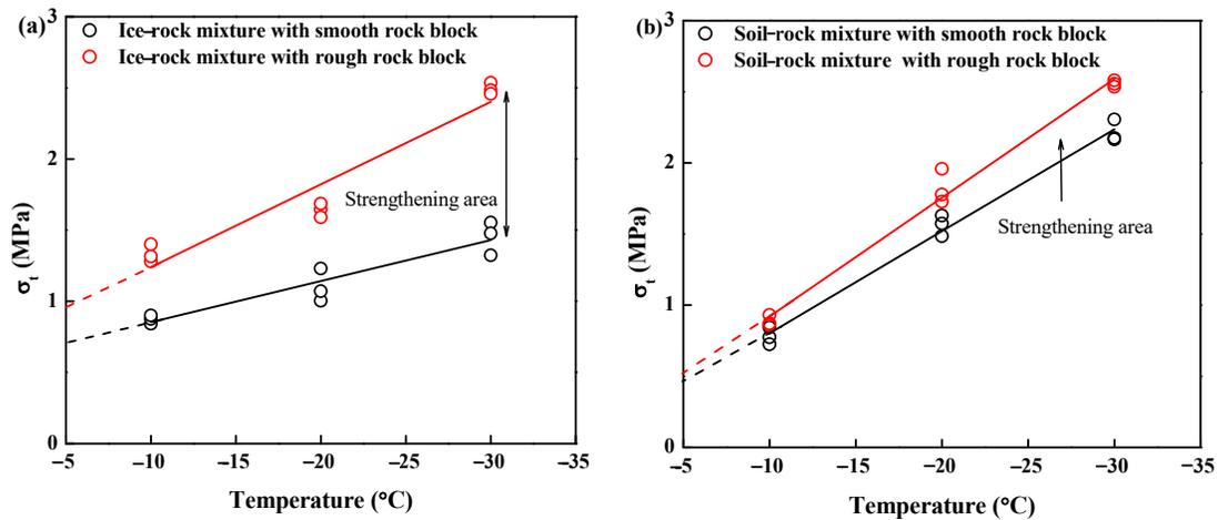
**Figure 13.** Relationship between indirect tension strength and frozen temperature (a) ice-rock mixture; (b) soil-rock mixture.
