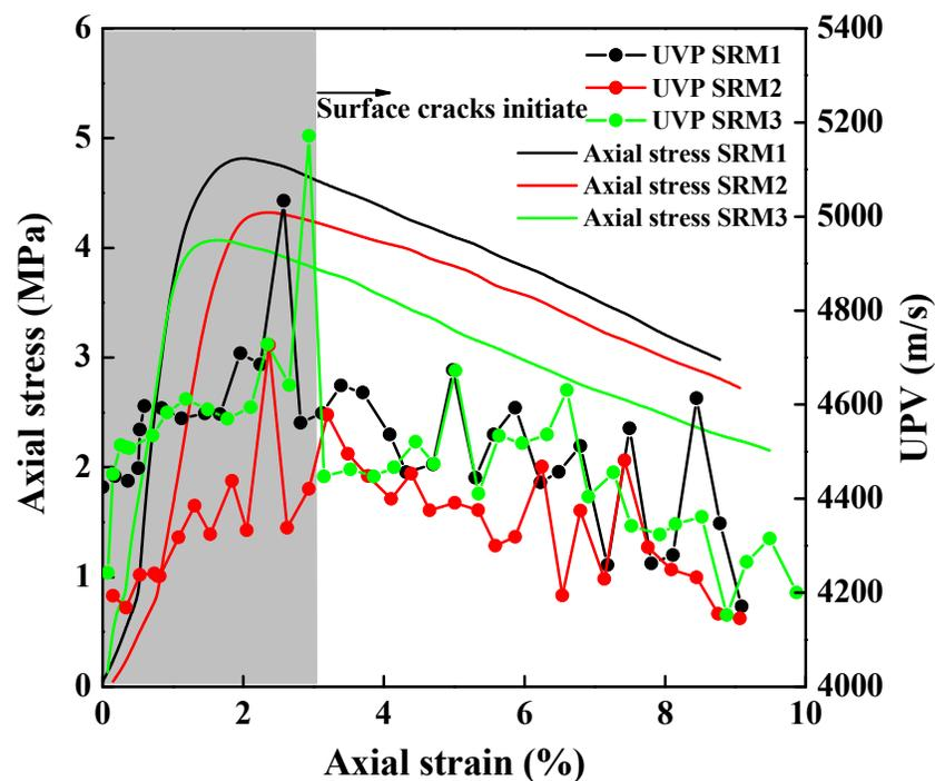
Figure 8. Relationship between the axial stress–strain and UPV.
