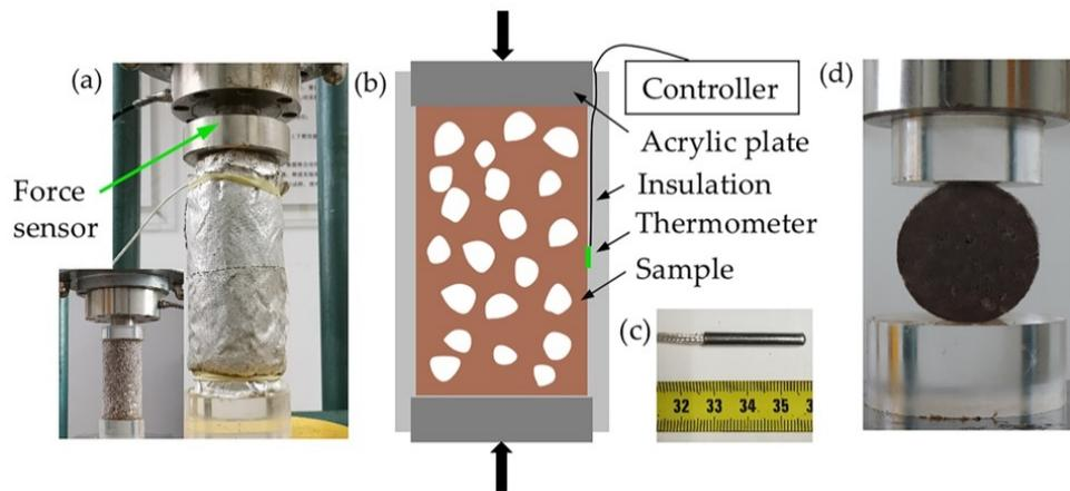
**Figure 3.** The testing apparatus and method: (a) uniaxial compression test; (b) sketch of the testing system; (c) thermometer probe; (d) Brazilian test.
