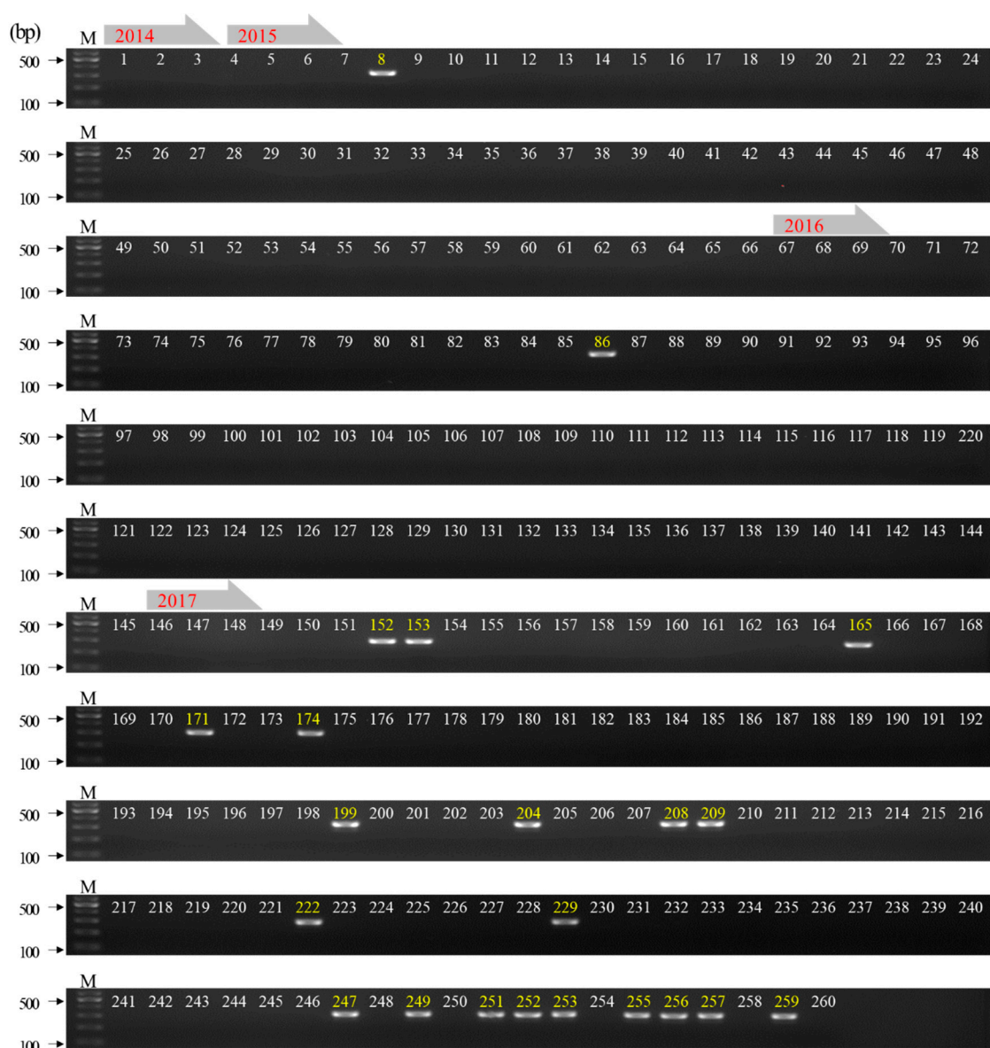
Figure 4. Application of the multiplex PCR method for living modified organism (LMO) identification with the collected suspicious canola samples. The numbers indicate the collection year of the suspicious canola samples (red) and are identified as LM canola (yellow).
