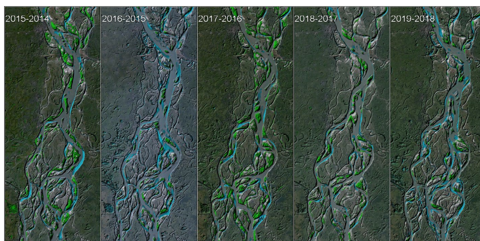
Figure 13. The satellite-derived differences for annual water occurrences computed using MoMo, showing deposition (green areas) and erosion (light-blue areas). Every image shows the difference
