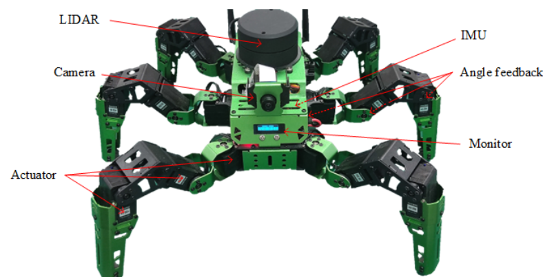
Figure 2. Structure of the hexapod robot.
