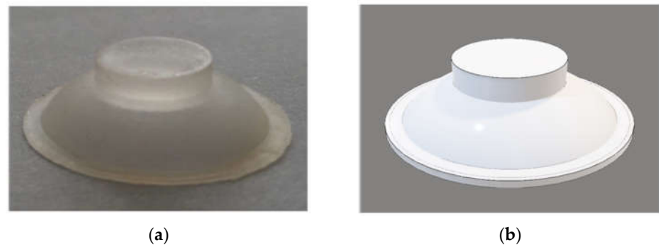
Figure 7. Fully polymeric dome: (a) real-life prototype; (b) 3D rendering implemented in COMSOL Multiphysics®.
