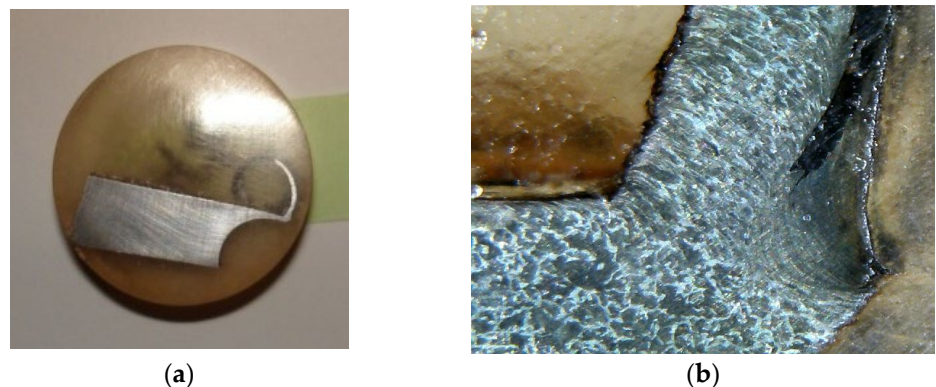
Figure 5. Investigated sample of a chip, (a) ground and polished, (b) etched, magnified 200 \times .
