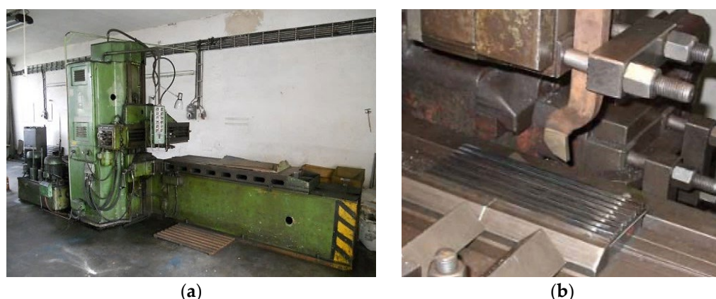
Figure 2. Experimental device (a) HJ8A planer, (b) experimental processing of a workpiece made of EN C45 steel.
