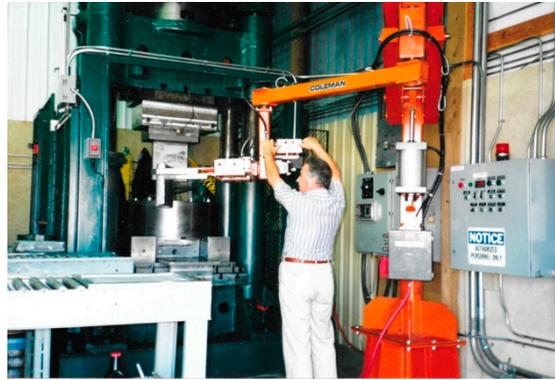
Figure 10. Billet loading in the die.
