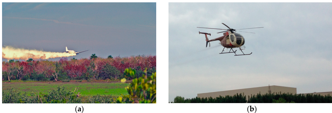
Figure 2. (a) An aerial adulticiding mission using fogging (Courtesy of G. Alan Curtis); (b) An aerial adulticiding mission using ultra-low volume (ULV) (Courtesy of Mark D. Latham).
