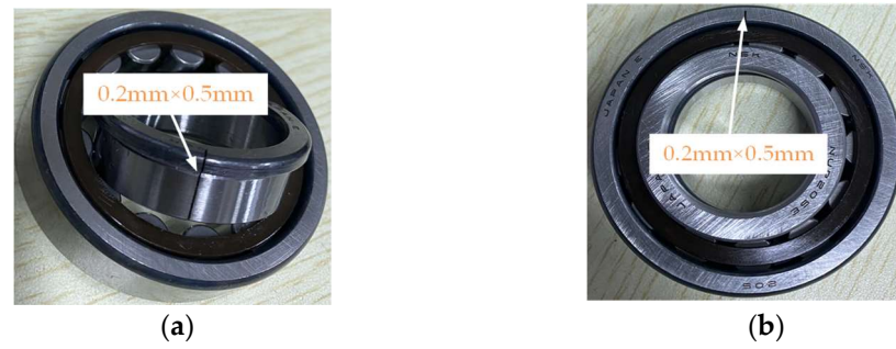
Figure 6. Defective bearings: (a) localized defects on inner ring; (b) localized defects on outer ring.
