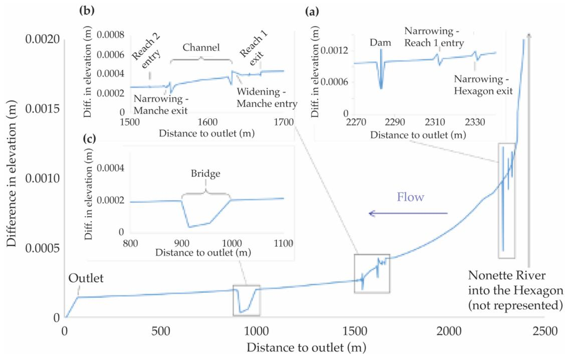
**Figure 13.** Calculated longitudinal profile of the deposition height downstream of the GC on 31 December 1987. (a) Details of the calculated longitudinal profile between the Hexagon exit and the dam. (b) Details of the calculated longitudinal profile in the vicinity of the Channel. (c) Details of the calculated longitudinal profile at the bridge.
