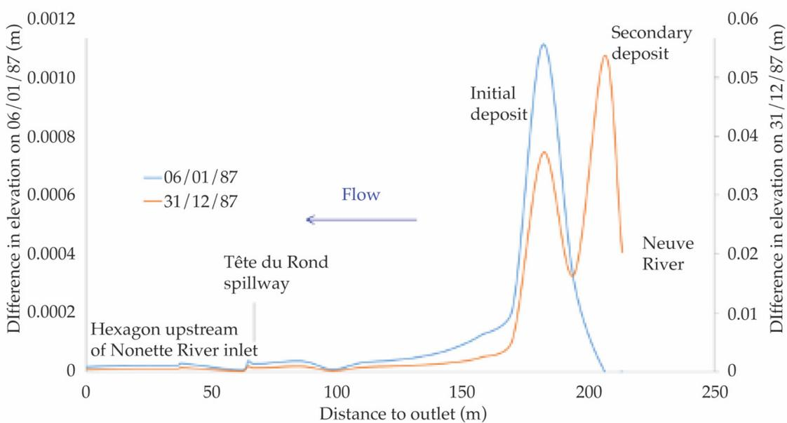
**Figure 12.** Calculated longitudinal profile of the deposition height upstream of GC on 6 January 1987.
