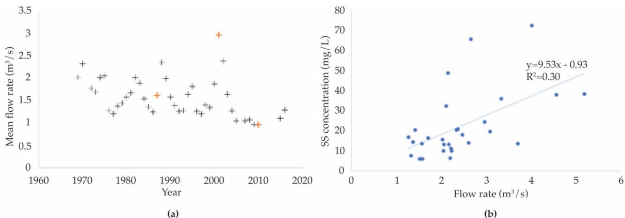
**Figure 9.** (a) Yearly mean flow rates from 1969 to 2016 [13]; red crosses show the typical years used for modelling. (b) Suspended solid concentrations as a function of the flow rate (values from [14,38,39]); linear regression used for modelling.
