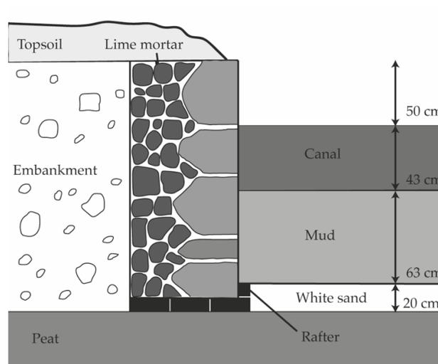
**Figure 8.** Structural scheme of GC walls, reproduced after [36].
