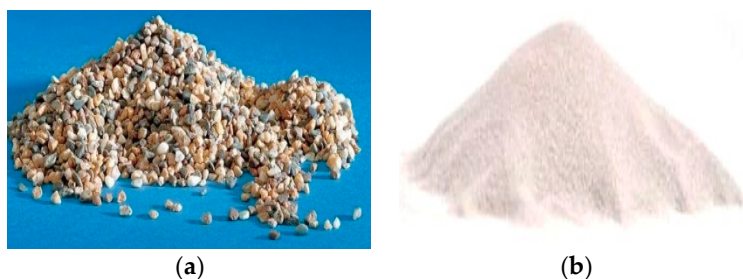
Figure 5. Materials used for the filter clogging: (a) fine gravel; (b) fine sand.
