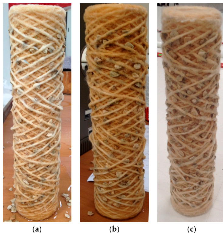
Figure 7. Progressive clogging rates of fine gravel: (a) 7.5%; (b) 15%; (c) 30%.
