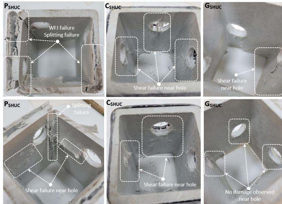
**Figure 6.** Damage analyses of  $P_{SHUC}$ ,  $C_{SHUC}$ ,  $G_{SHUC}$ .
