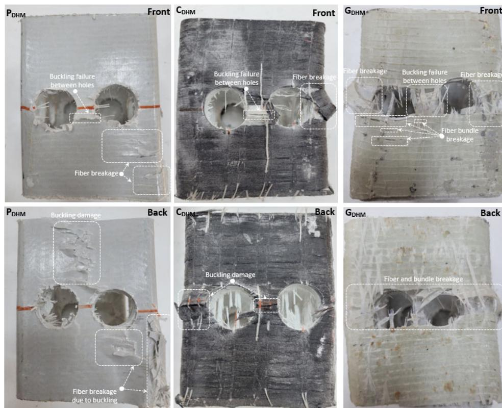
**Figure 8.** Damage analyses of  $P_{DHM}$ ,  $C_{DHM}$ , and  $G_{DHM}$ .
