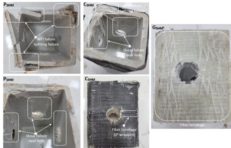
Figure 4. Damage analyses of P<sub>SHM</sub>, C<sub>SHM</sub>, G<sub>SHM</sub>.
