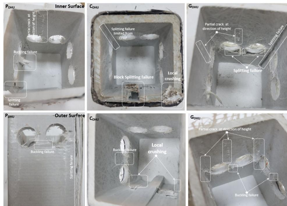
**Figure 9.** Damage analyses of  $P_{DHU}$ ,  $C_{DHU}$ , and  $G_{DHU}$ .
