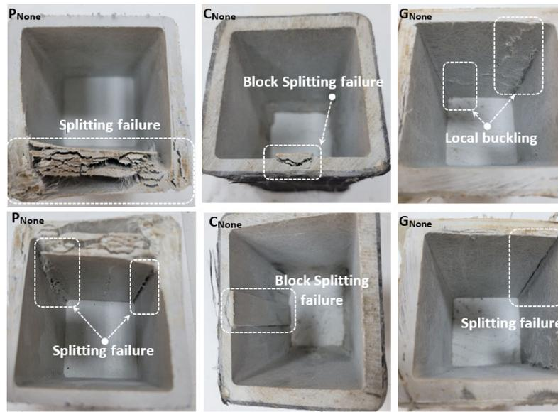
Figure 3. Damage analyses of PNone, CNone, GNone.
