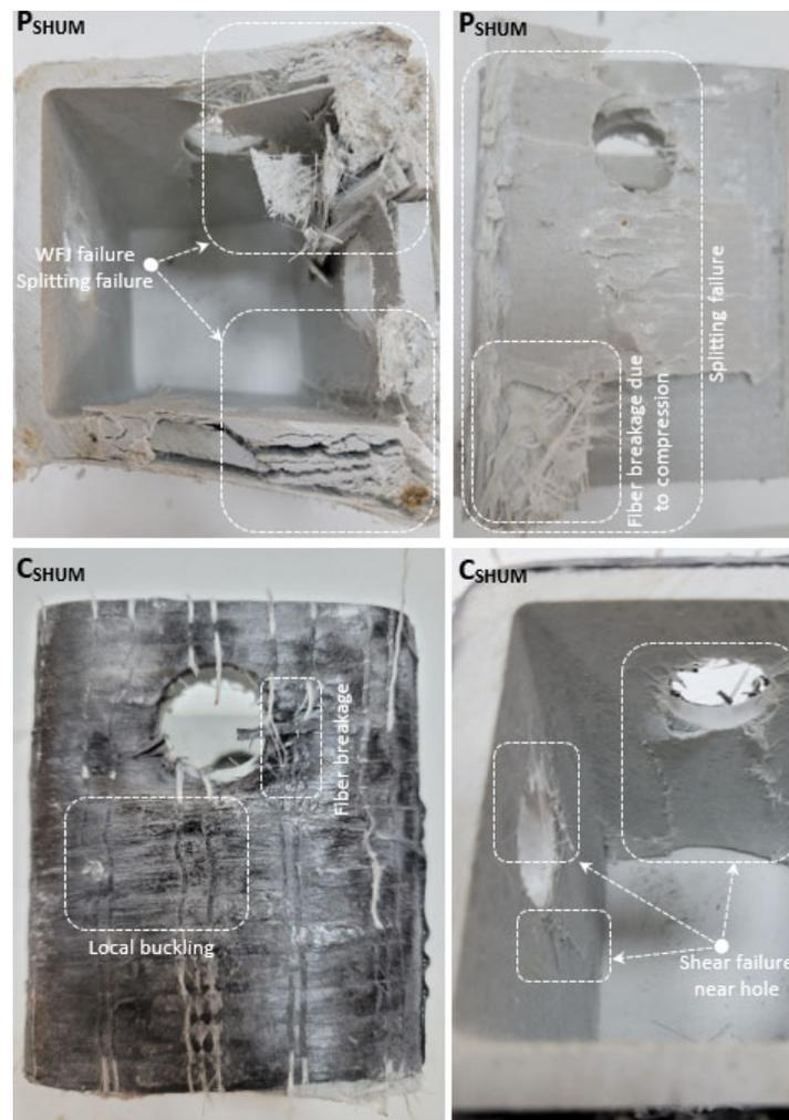
**Figure 7.** Damage analyses of  $P_{SHUM}$ ,  $C_{SHUM}$ ,  $G_{SHUM}$ .
