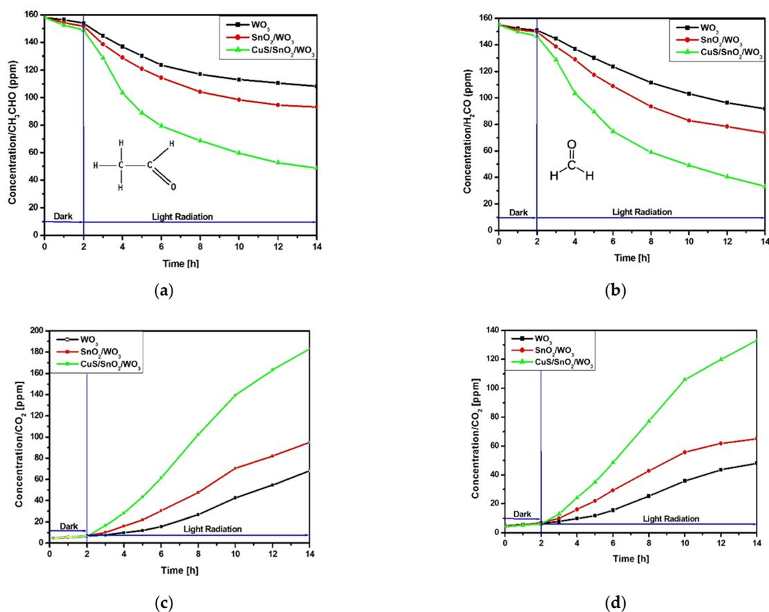
**Figure 4.** Photocatalytic removal of (a) acetaldehyde and (b) formaldehyde, and CO<sub>2</sub> evolution from (c) acetaldehyde and (d) formaldehyde degradation.
