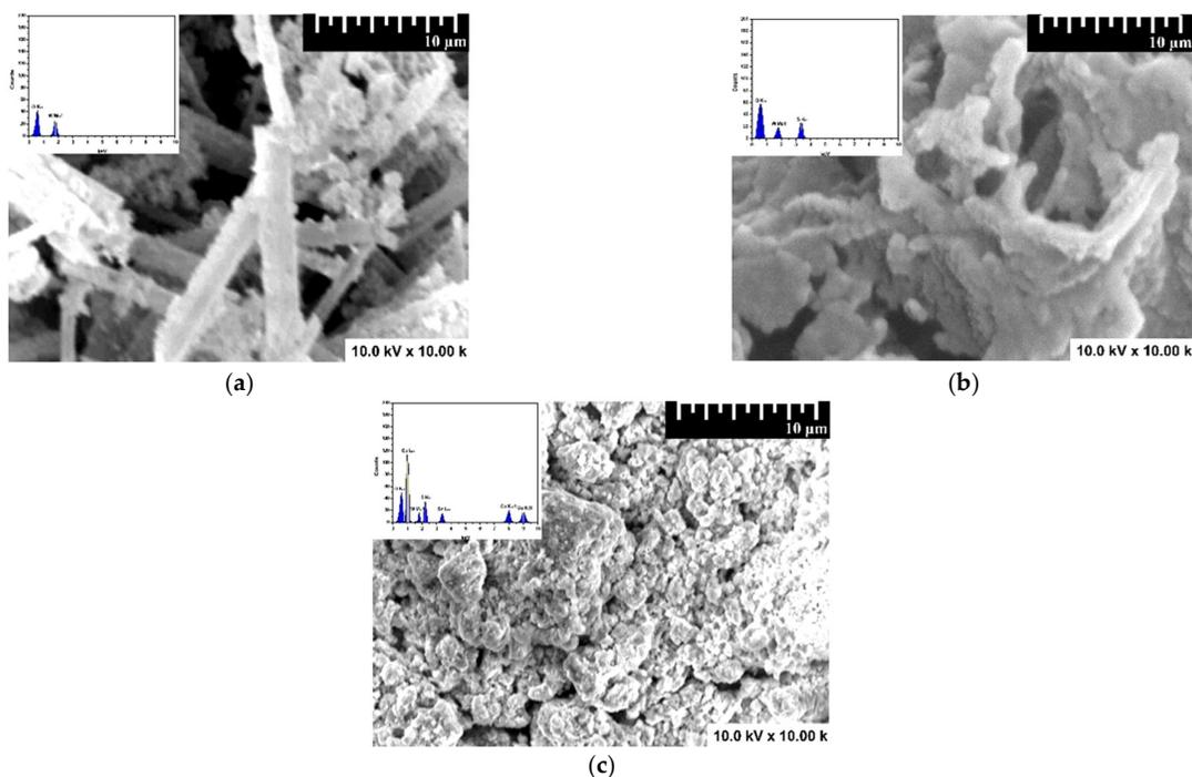
**Figure 2.** SEM pictures of the photocatalysts: (a) WO<sub>3</sub>, (b) SnO<sub>2</sub>/WO<sub>3</sub> and (c) CuS/SnO<sub>2</sub>/WO<sub>3</sub> (inset EDX spectra).
