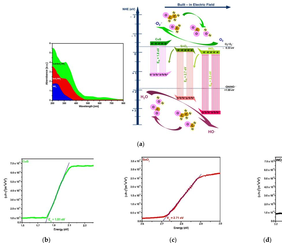
**Figure 7.** Heterostructure mechanism and absorption (a), and components band gap values (b–d).
