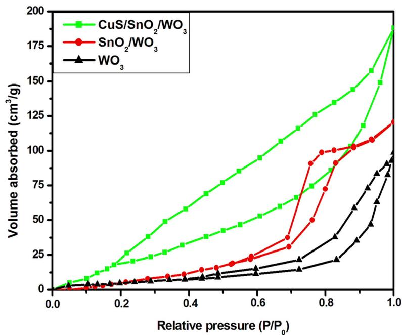
**Figure 3.** N<sub>2</sub> adsorption–desorption isotherm.
