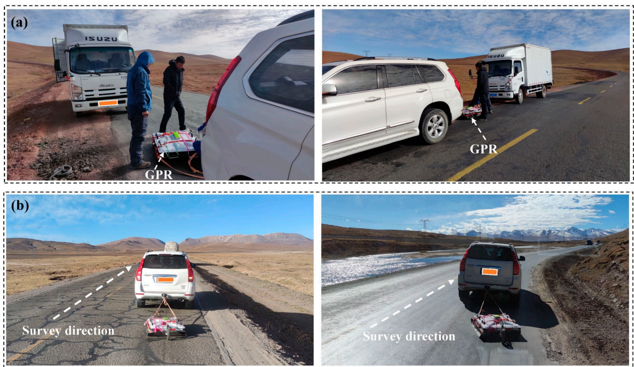
Figure 6. Diagram of the field GPR survey on QTH: (a) GPR survey system; (b) site survey.
