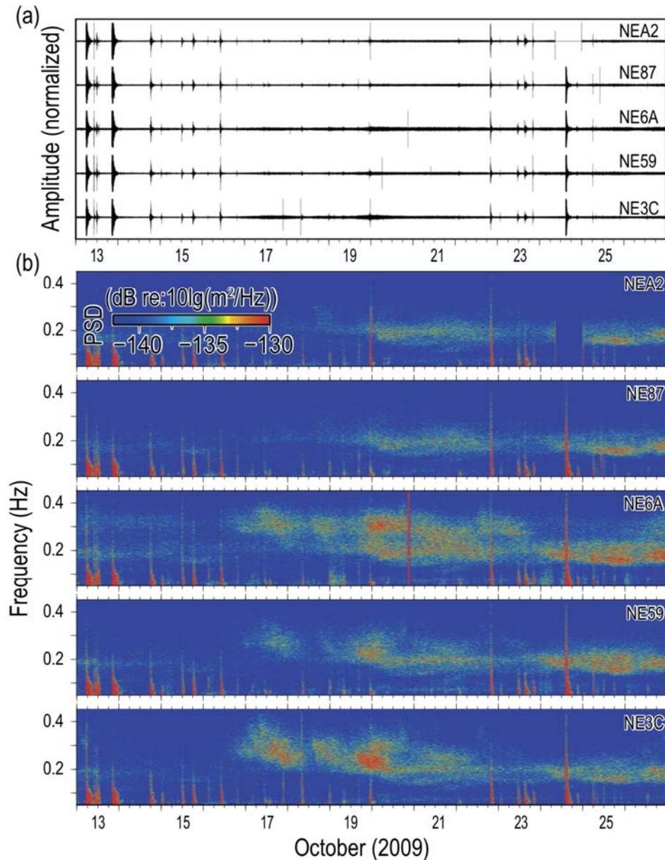
**Figure 2.** (a) Seismic waveforms and (b) temporal frequency spectrograms of the microseisms generated during the life span of typhoon Lupit at the stations NEA2, NE87, NE6A, NE3C and NE59 of NECESSArray, labeled by blue triangles in Figure 1. The unit (dB) corresponds to  $10 \cdot \log_{10}(\text{m}^2/\text{Hz})$ .
