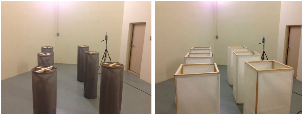
Figure 5. Pictures of the experimental setups. The left figure includes 1 m 2 CPMSA made of membrane A, and the right figure includes 2 m 2 RPMSA made of membrane C.
