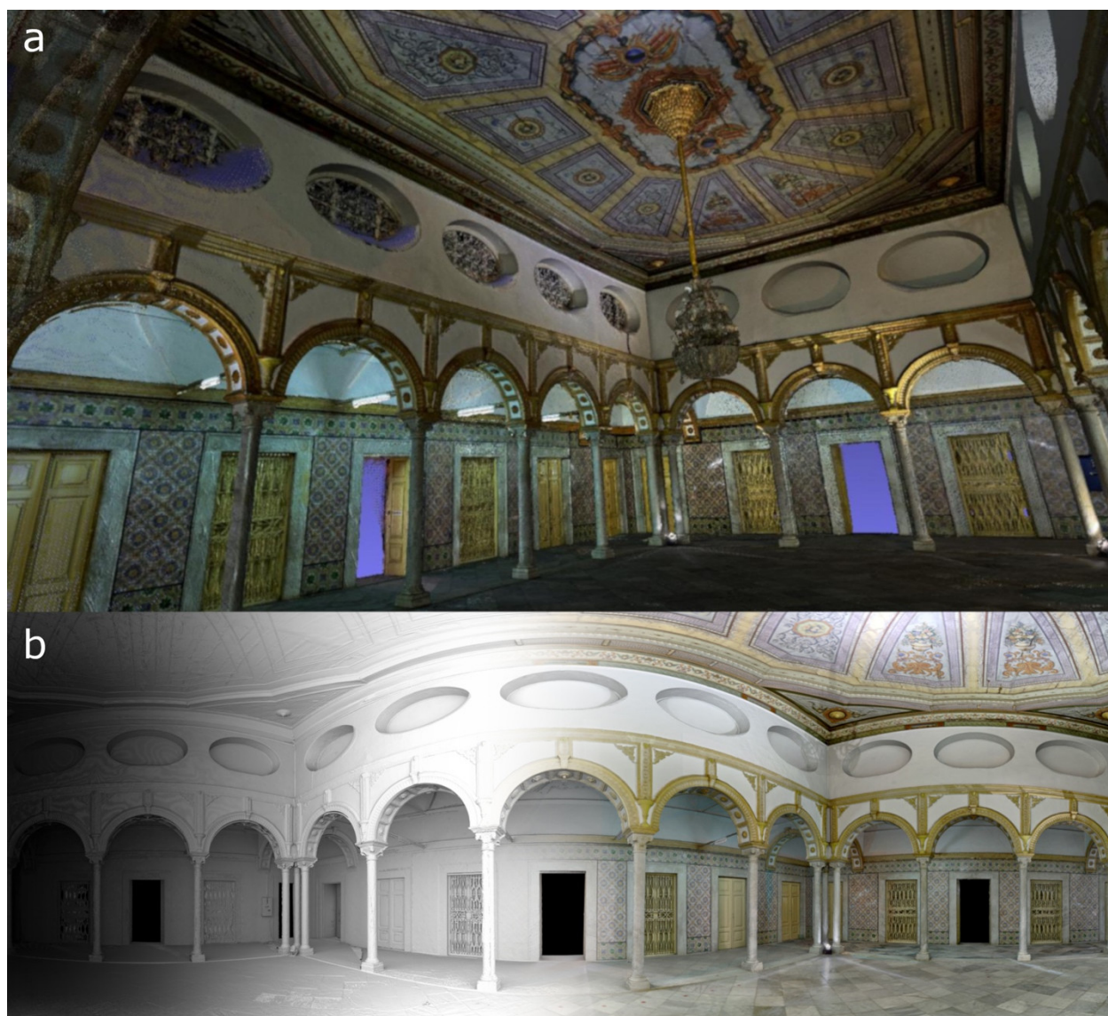
Figure 2. Laser scanning 3D model of the Ksar Said main salon: (a) Point cloud 3D model; (b) Textured 3D model.
