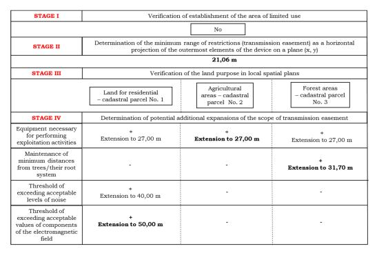
Figure 2. Determination of the range of transmission easement for the model object.
