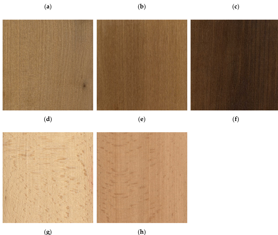
Figure 6. (a) Untreated birch, (b) birch treated at 160 °C, (c) birch treated at 170 °C, (d) birch treated at 180 °C, (e) birch treated at 190 °C, (f) birch treated at 200 °C, (g) untreated beech, (h) steamed beech.
