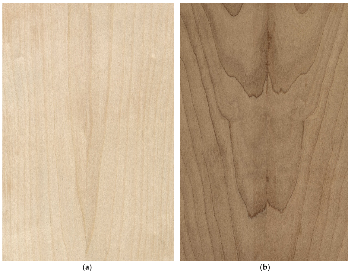
Figure 12. (a) Sample of untreated birch veneer. (b) Sample of treated veneer under a temperature of 200 °C for 2 hours.
