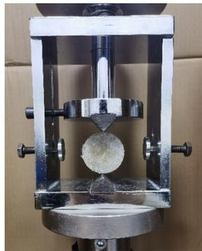
**Figure 5.** Splitting tensile test angular fixture.
