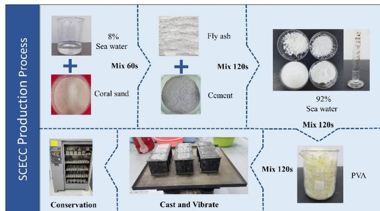
**Figure 2.** Fabrication process of SCECC specimens.
