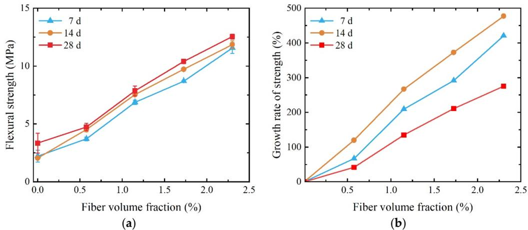
**Figure 11.** Three-point bending strength of SCECC with different fiber content and ages: (a) three-point bending strength; (b) the growth rate of strength.
