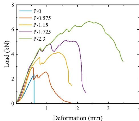
**Figure 14.** Splitting tensile load–deformation curves of SCECC.
