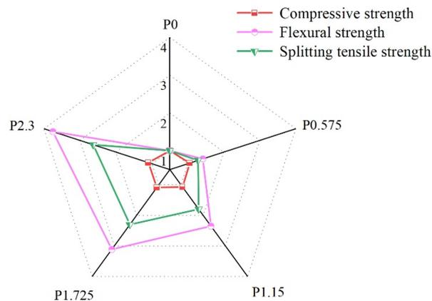
**Figure 16.** Mechanical properties of PVA fiber reinforced the vertical coordinates in the graphs representing the multiplicative increase in compressive, three-point flexural, and split tensile strengths of the various specimen groups relative to the P-0 group.
