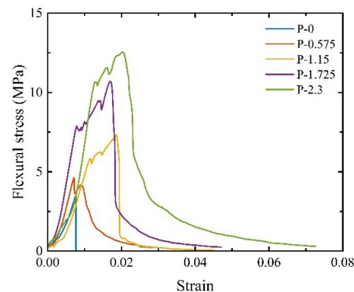
**Figure 9.** Three-point bending stress–strain curves of SCECC.
