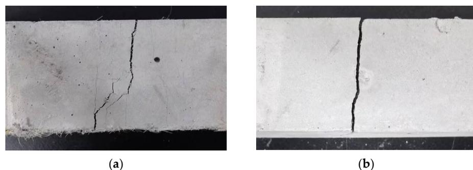
**Figure 10.** Failure mode of the three-point bending test specimen: (a)  $V_f = 1.725\%$ ; (b)  $V_f = 0\%$ .
