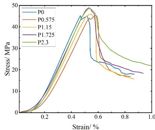
**Figure 6.** Uniaxial compressive stress–strain curves of SCECC.
