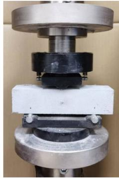
**Figure 4.** Three-point bending test loading device.
