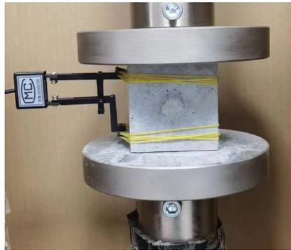
**Figure 3.** Compressive strength test specimen.
