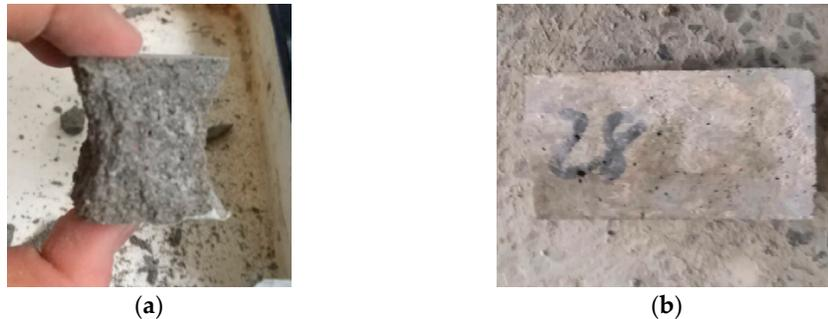
**Figure 2.** Compressive and flexural failure specimens. (a) Compressive failure specimen and (b) flexural failure specimen.
