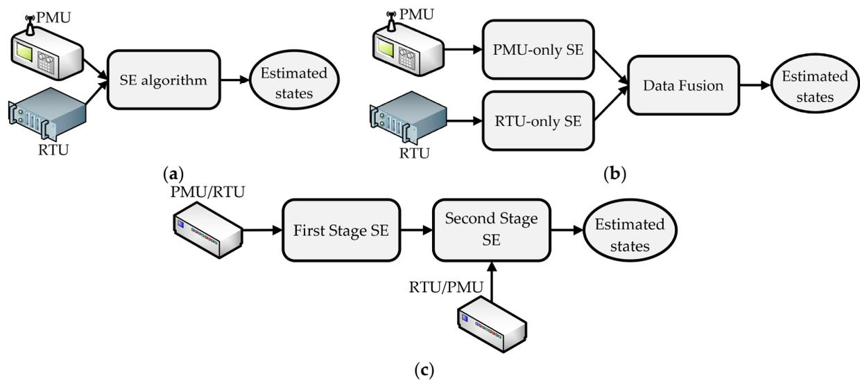
**Figure 4.** Typical structure of HSSE methods: (a) One-Stage HSSE; (b) Fusion HSSE; (c) Two-Stage HSSE.
