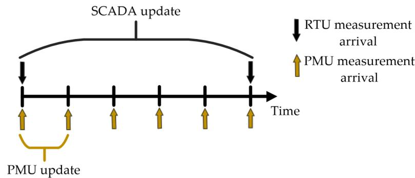
**Figure 3.** The dissimilarity between RTU and PMU measurement refresh rates.
