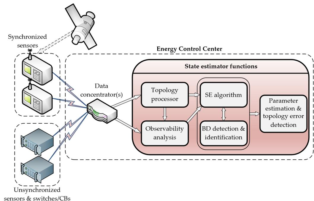
**Figure 1.** Data flow diagram of SE, from the field sensors to the ECC.
