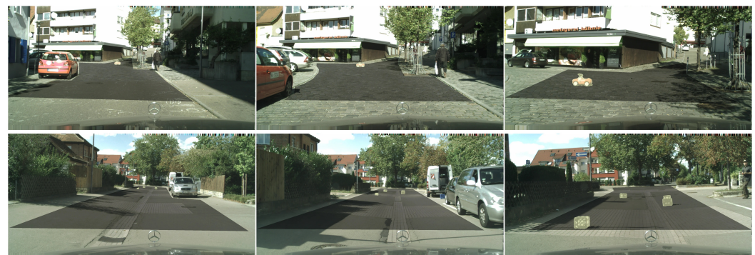
Figure 6. OOD detection on LostAndFound dataset. Our method can detect obstacles at different distances from the camera ( top ) as well as multiple obstacles in one image ( bottom ). The road ground truth is designated in grey and the predicted OOD in yellow. Zoom in to see the distant obstacles.
