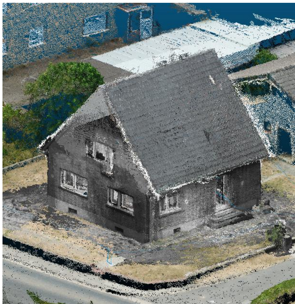
Figure 10. Complementary 3D reconstruction from UAV imagery (colored parts inclusive of the gray roof) combined with IPS on-ground derived point cloud (ground surroundings and building walls shown in grayscale).
