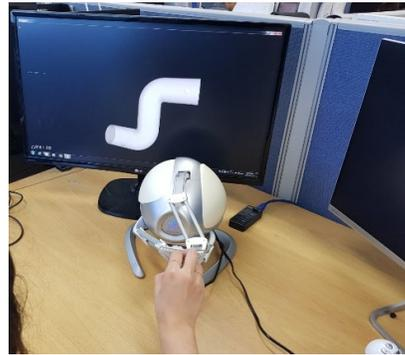
**Figure 2.** Upper limb rehabilitated by catching the haptic probe and passing through the three-dimensional rehabilitation model.
