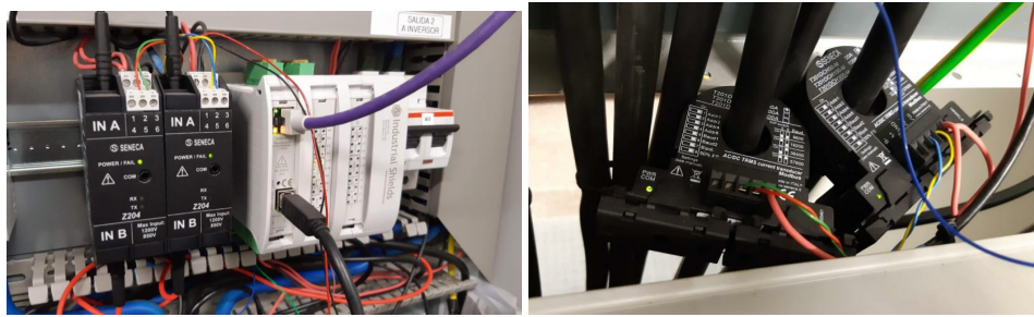
Figure 3. Current and voltage sensors and microprocessor unit. (a) Two voltage sensor devices for the two branch of the generator under study (black units) and the \mu P unit (white one); (b) Two current sensor, toroidal cores, for the two branch of the generator under study.
