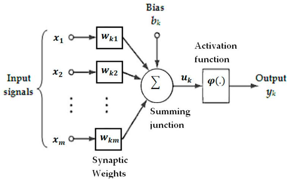
Figure 3. An artificial neuron model structure [78].
