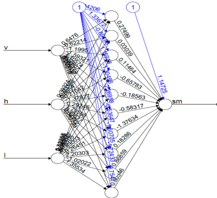
**Figure 4.** Artificial neural network (ANN) architecture used for soil moisture estimation using  $v - \sigma_{soil_{vv}}$ ,  $h - h_{rms}$ , and  $l - l_{eff}$  as input variables and soil moisture (sm) as the output variable. The structure has one hidden layer and 10 hidden neurons.
