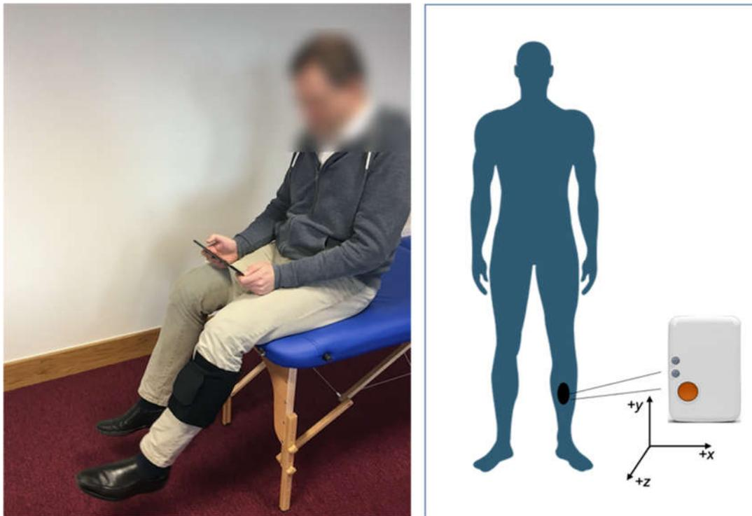
**Figure 1.** User setup and IMU orientation of the biofeedback system consisting of a single IMU and associated Android tablet application (figure adapted from [23]).
