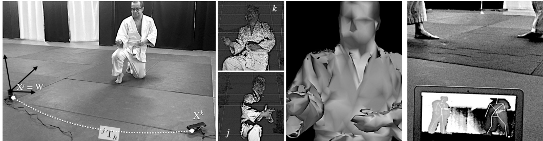
Figure 5. Leftmost images: Two spatially registered depth sensors of ASUS and Microsoft, respectively—corresponding point clouds as measured from both devices and low-quality textured-mesh isosurface reconstruction. Rightmost image: OpenNI-compatible sensor (placed behind the laptop's screen and not visible in the photographs) that track the movement of two aikido practitioners ( shomen-uchi kotegaeshi ). Their skeletons are derived in real-time and appear in the laptop's screen. Images correspond to one of the co-authors of the paper and were obtained at Judelda dojo (Elda, Spain).
