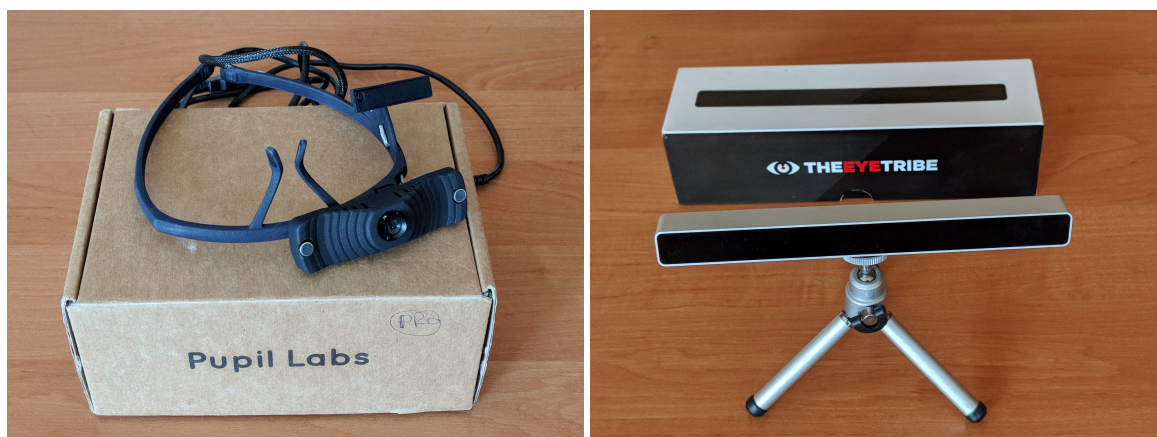
Figure 6. Eye trackers used during the experimental part of the research. Left: Pupil Labs headset eye tracker, right: The Eye Tribe remote eye tracker to be mounted below a screen.
