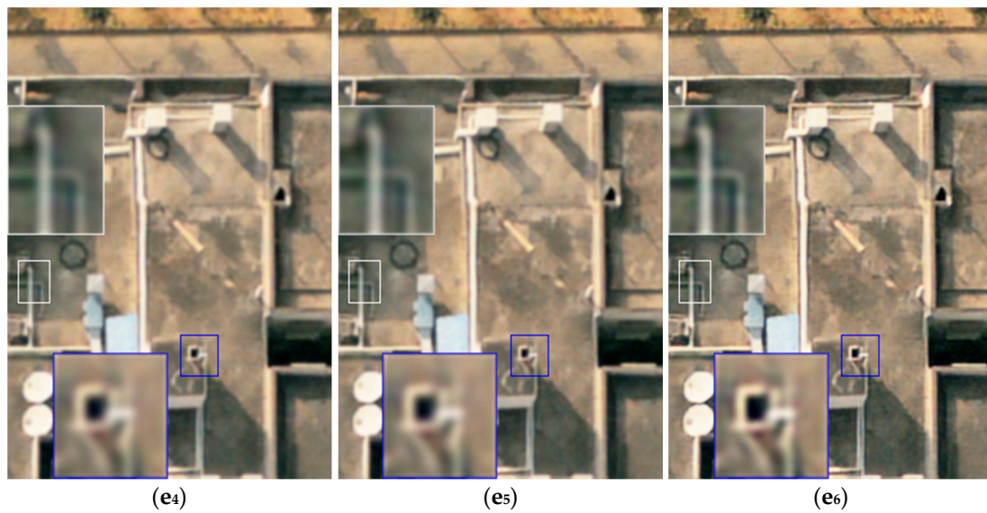
Figure 2. Testing results of several denoising methods for UAV images with several ground objects. In each group of images, the 1st image ( a_1, b_1, c_1, d_1, e_1 ) is the ground truth; the 2nd image ( a_2, b_2, c_2, d_2, e_2 ) is a noise image with noise level 35; and the 3rd image ( a_3, b_3, c_3, d_3, e_3 ) presents the denoising results of method [8]. The 4th image ( a_4, b_4, c_4, d_4, e_4 ) presents the denoising results of method [5]; the 5th image ( a_5, b_5, c_5, d_5, e_5 ) presents the denoising results of method [17]; and the 6th image ( a_6, b_6, c_6, d_6, e_6 ) presents the denoising results of the proposed method.
