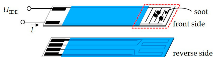
Figure 1. Sketch of the sensor setup: The sensors front side comprises interdigital electrodes (IDE) where soot deposits yield electrical conductive pathways over the spacing. On the reverse side, a four-wire thick-film heater allows temperature-controlled sensor regeneration as well as temperature measurement and temperature adjustment during soot deposition.
