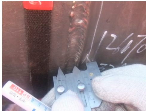
Figure 5. Profile of a mismatched weld joint.
