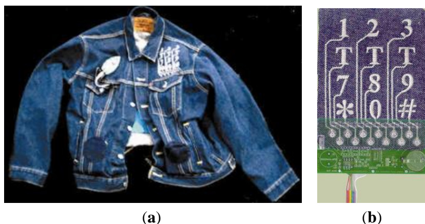
Figure 8. (a) Musical Jacket comprising a fabric keypad on one side, a MIDI synthesizer on the other side, speakers behind speaker grills in the pockets and fabric buses visible inside the jacket; (b) The fabric keypad with the circuit board placed behind it.
