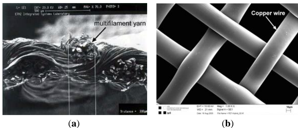
Figure 20. SEM image of fabric with copper fiber (a) and PETEX (b).
