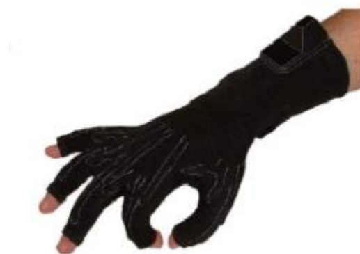
Figure 11. DataGlove™ VRLOGIC with flex sensors.
