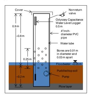
**Figure 4.** Groundwater piezometer for water sampling and monitoring of groundwater table depths. Each piezometer is equipped with a sampling pump, nonreturn valve and capacitance water logger.
