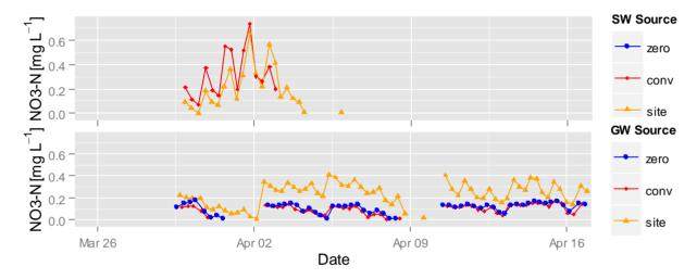
**Figure 9.** Relative SW (**top**) and GW (**bottom**) levels from the end of March to mid-April at the site-specific fertilized plot. The strong increases in SW level are irrigation events. The regular fluctuation in the GW is given due to pumping and refilling of the piezometer.
