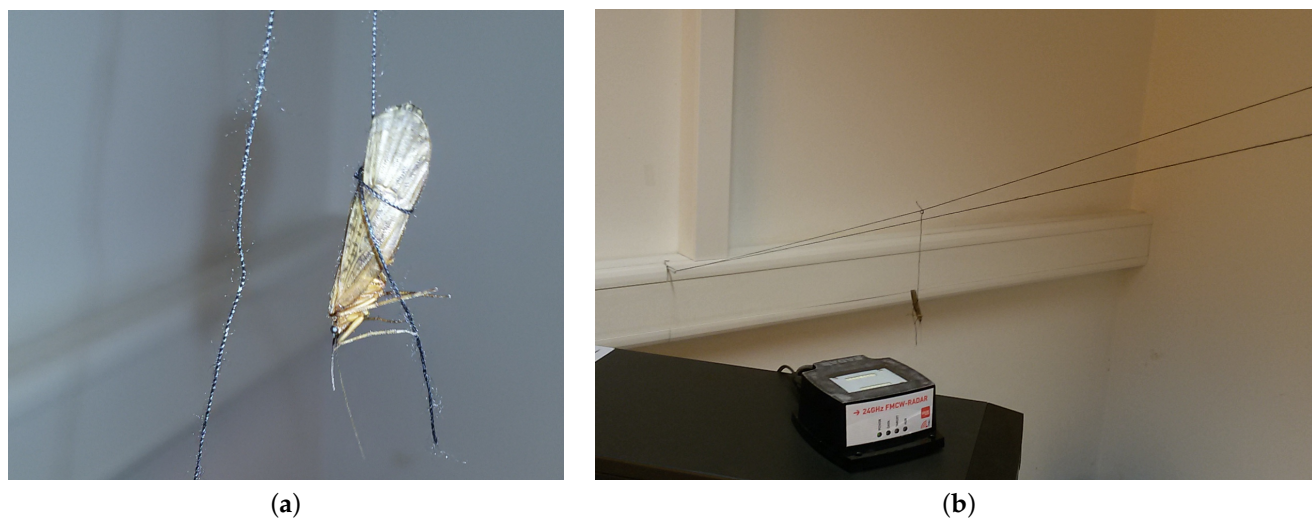
Figure 2. Phryganea grandis : (a)—tied with a thread, (b)—placed above the radar.
