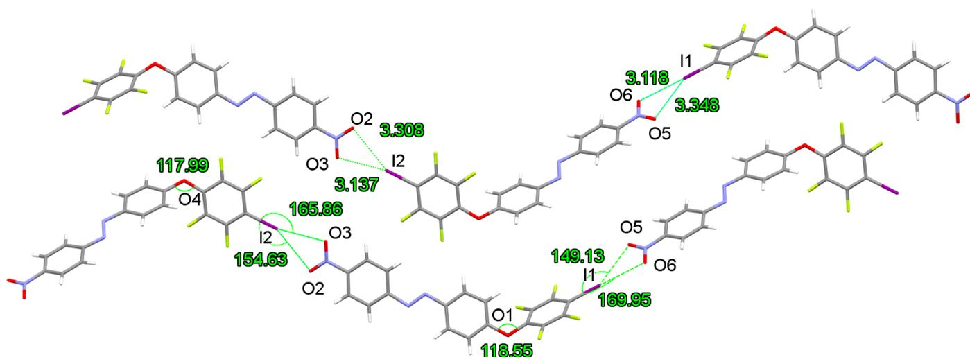
**Figure 1.** X-ray structure of I-azo- $\text{NO}_2$  developing undulating parallel chains due to two  $\text{O} \cdots \text{I}$  halogen bonds. Colors are as follows: grey, C; blue, N; red, O; white, H; yellow, F; purple, I.  $\text{O} \cdots \text{I}$  bond distances (Å) and  $\text{C}-\text{I} \cdots \text{O}$  bond angles ( $^\circ$ ).
