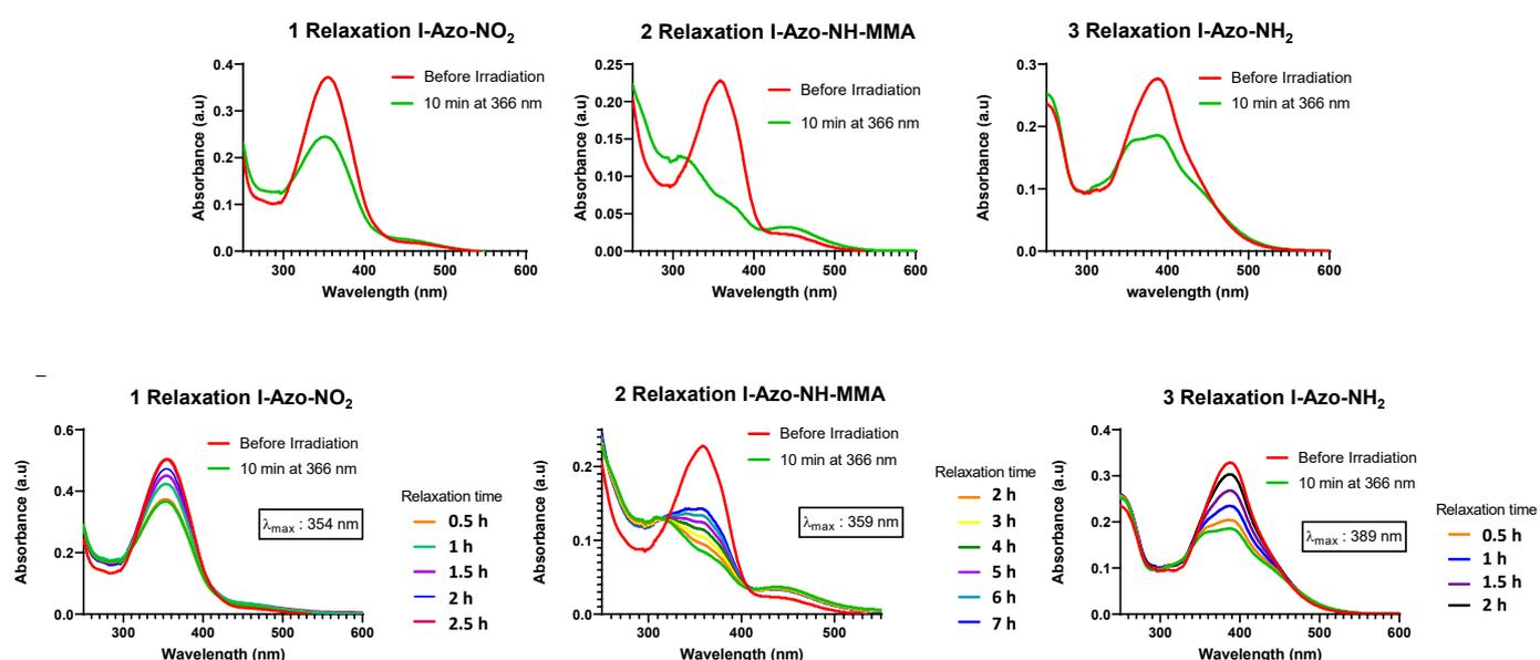
**Figure 5.** UV-Vis spectra for I-azo-NO<sub>2</sub> (A1), I-azo-NH-MMA (A2) and I-azo-NH<sub>2</sub> (A3) before (red) and after (green) a 10 min exposure to 366 nm light. Thermal relaxation spectra in the dark for I-azo-NO<sub>2</sub> (B1), I-azo-NH-MMA (B2) and I-azo-NH<sub>2</sub> (B3).
