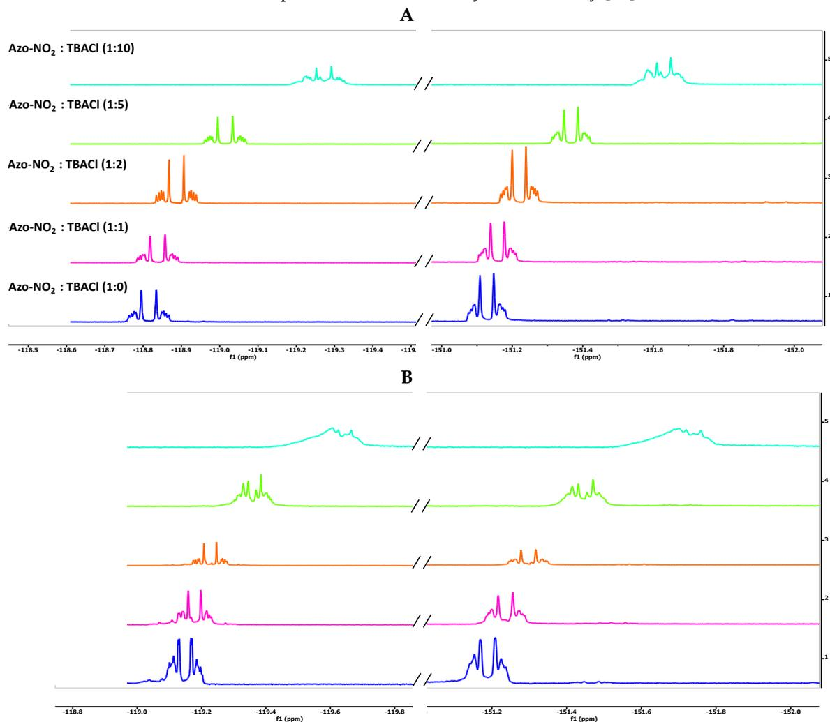
**Figure 4.** Stack plot of <sup>19</sup>F-NMR spectra of I-azo-NO<sub>2</sub> and I-azo-NH-MMA (CDCl<sub>3</sub>), at different molar ratios of I-azo-NO<sub>2</sub>/TBACl (A) and I-azo-NH-MMA/TBACl (B). Molar ratios: a) 1:0; b) 1:1; c) 1:2; d) 1:5; e) 1:10.
