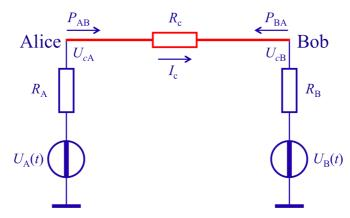
The signal inherent in the Second-Law-attack scales linearly with  $R_c$ , which provides a much better situation for Eve—especially in the case of vanishing cable resistance—than the square-law scaling of the BSY attack. Moreover, it is also obvious that in a practical case [3,9,10], where  $R_c \ll R_L \ll R_H$ , Eve's signal-to-noise ratio is always greater in the Second-Law-attack than in the BSY attack. This is
